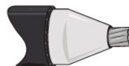
PENCILING INSULATION ON URD CABLE
