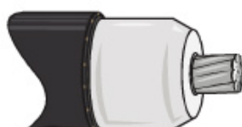
CHAMFERING INSULATION ON URD CABLE END
