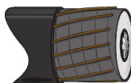
STRIPPING URD CABLE JACKET
