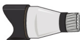
PENCILING INSULATION ON TRANSMISSION CABLE
