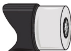
STRIPPING SEMI-CON FROM URD CABLE
