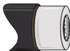
SHAVING SEMI-CON FROM TRANSMISSION CABLE
