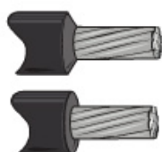
STRIPPING END OF SECONDARY CABLE TO SQUARE OR CHAMFER
